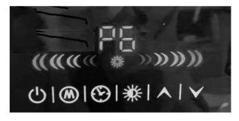
button. The unit will revert back to showing the standby "P0" screen. 5.9. To power off the unit, use the
